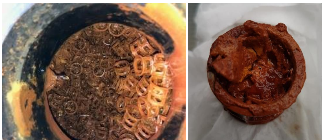
Figure 4. 19 Packing material of the tower aerator
