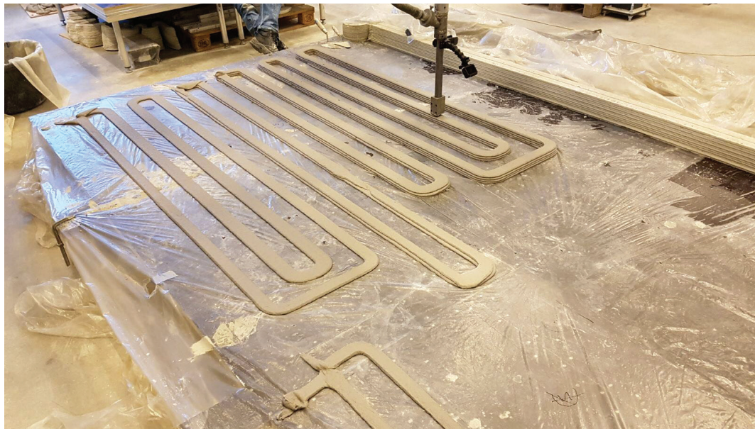
FIGURE 3 Printing with one of the developed PVA-fiber reinforced Strain Hardening Cementitious Composites.
