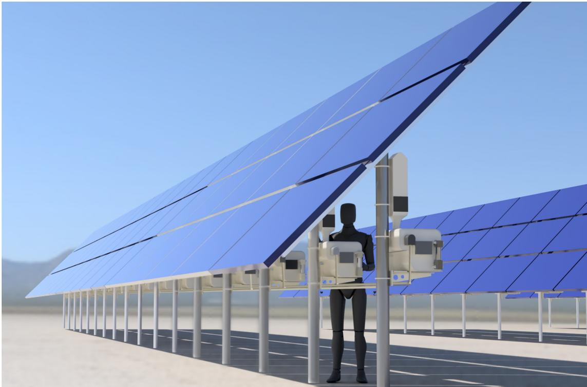
*Figure 1.2:* A visual of the ZEF micro-plant relative to the size of a human person. The micro-plant farm will consist of many rows of multiple ZEF micro-plant units (40,000 units). Image by courtesy of David van Nunen.
