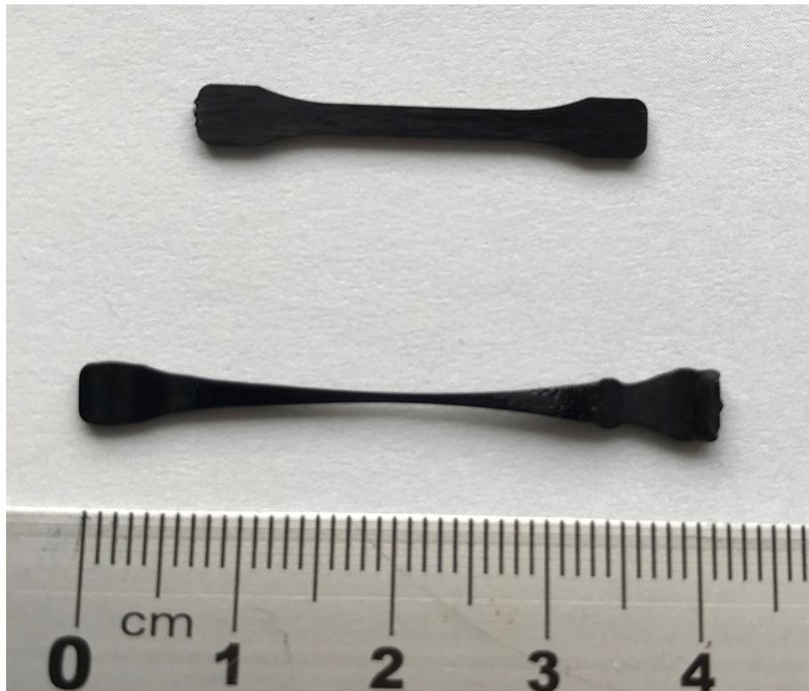
Figure 6.8: Image of a PSU sample after performing a DMA test.
