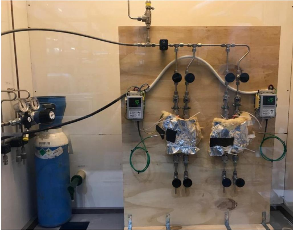
Figure 4.2: Setup of accelerated ageing system
