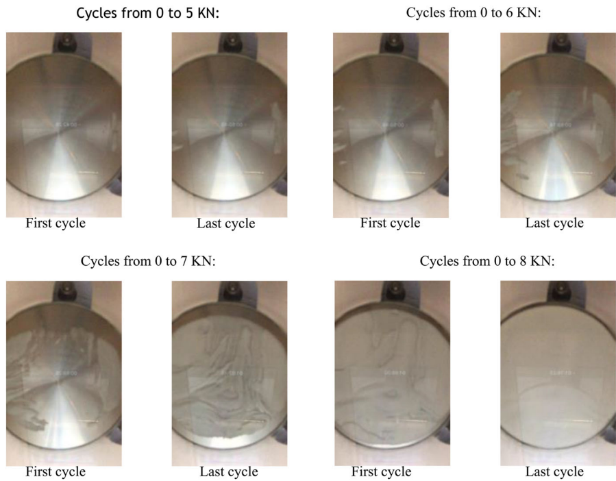
Fig. 16 Whitening effect propagation under loading cycles
