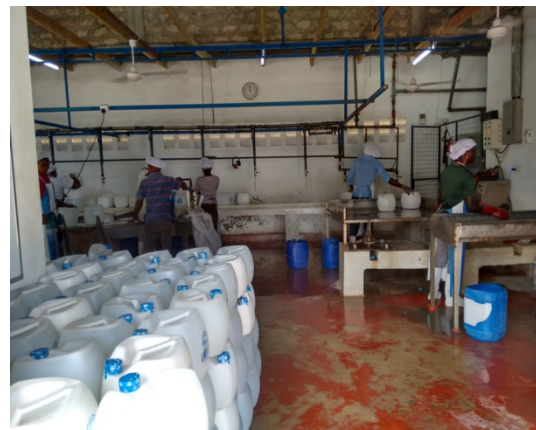
Figure 2: Cleaning process for 10L reusable jerry cans
