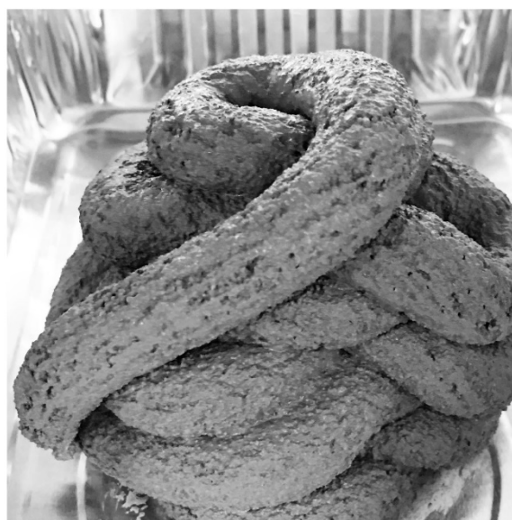
Figure 8. (a) Extruded filaments of mixtures MIX-1, MIX-2, and MIX-3 at different ages. The images with the red frame represent that the extruded filaments have a relatively weak shape stability, compared with others. The shape stability was evaluated by visual inspection. (b) An example of a relatively weak shape stability (MIX-3 at the age of 10 min). (c) An example of a good shape stability (MIX-1 at the age of 10 min).
