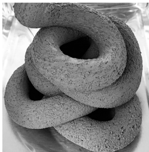
Figure 8. (a) Extruded filaments of mixtures MIX-1, MIX-2, and MIX-3 at different ages. The images with the red frame represent that the extruded filaments have a relatively weak shape stability, compared with others. The shape stability was evaluated by visual inspection. (b) An example of a relatively weak shape stability (MIX-3 at the age of 10 min). (c) An example of a good shape stability (MIX-1 at the age of 10 min).
