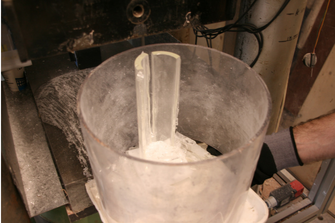
Figure 111: remainder after a test, still visible are the long cracks over the entire height of the sample ultimately leading to complete failure
