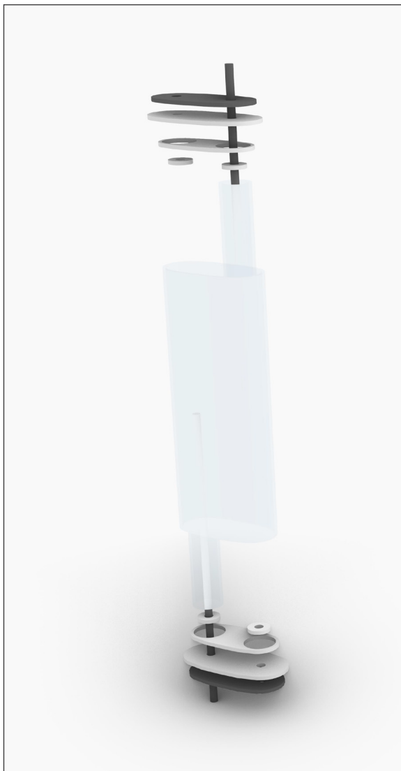
Figure 32: exploded view of the preliminary design, length of the glass segments is shortened for this image
