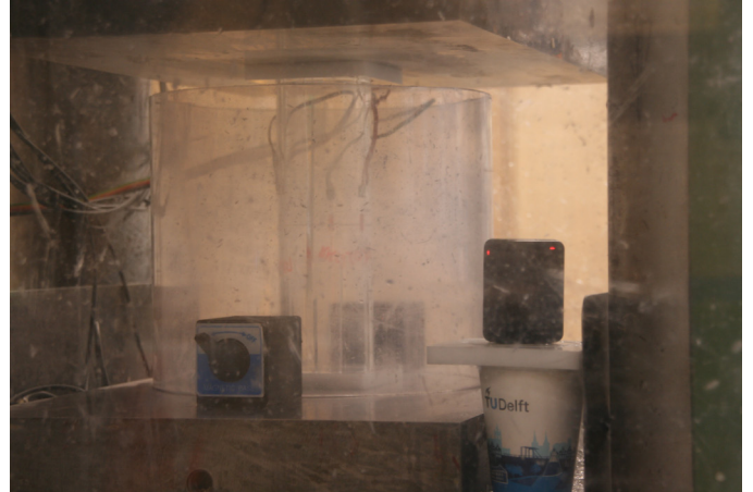
Figure 100: the tube for catching shrapnel was held in place by magnets and most experiments could be filmed
