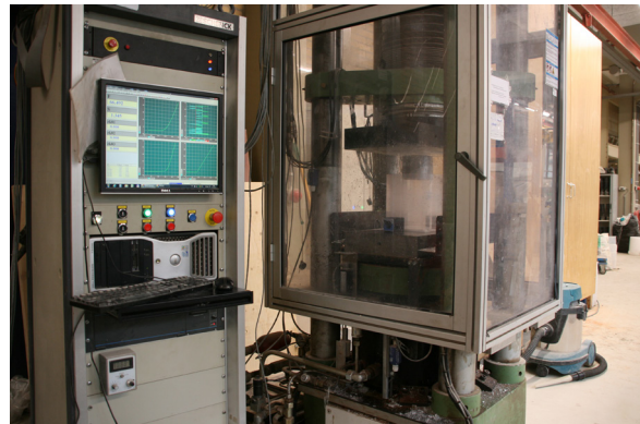
Figure 56: the Toni-bank used for the compressive tests
