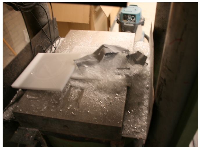
Figure 115: remainder of sample after a test, leaving a lot of shrapnel
