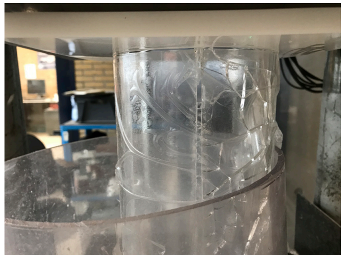
Figure 114: a crack along the entire height of the profile splits the section
