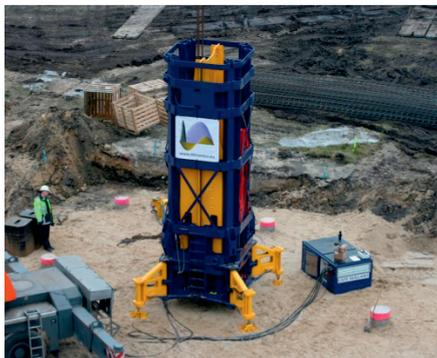
(a) Rapid pile load test 8MN [188]
