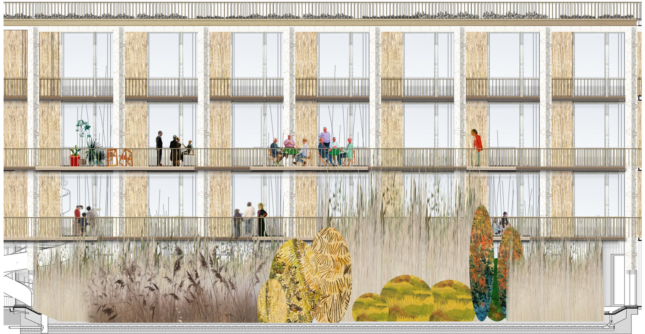
Impression of Bioretention reed garden Apart from a water catchment area, it also adds quality to the overall space.
