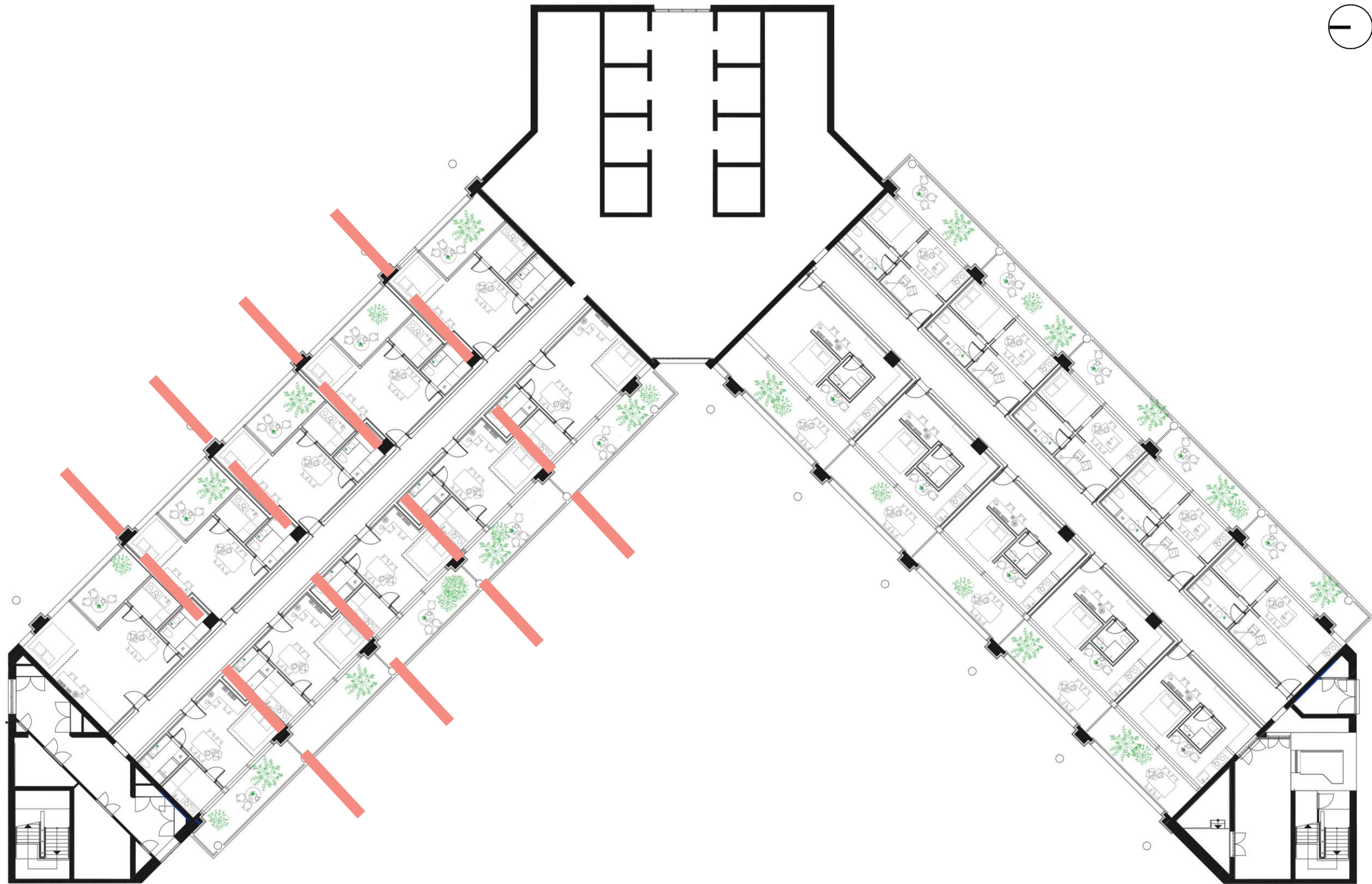
Typical Floor Plan B. Level 3 Unit division staggered off from grids. Scale 1:250
