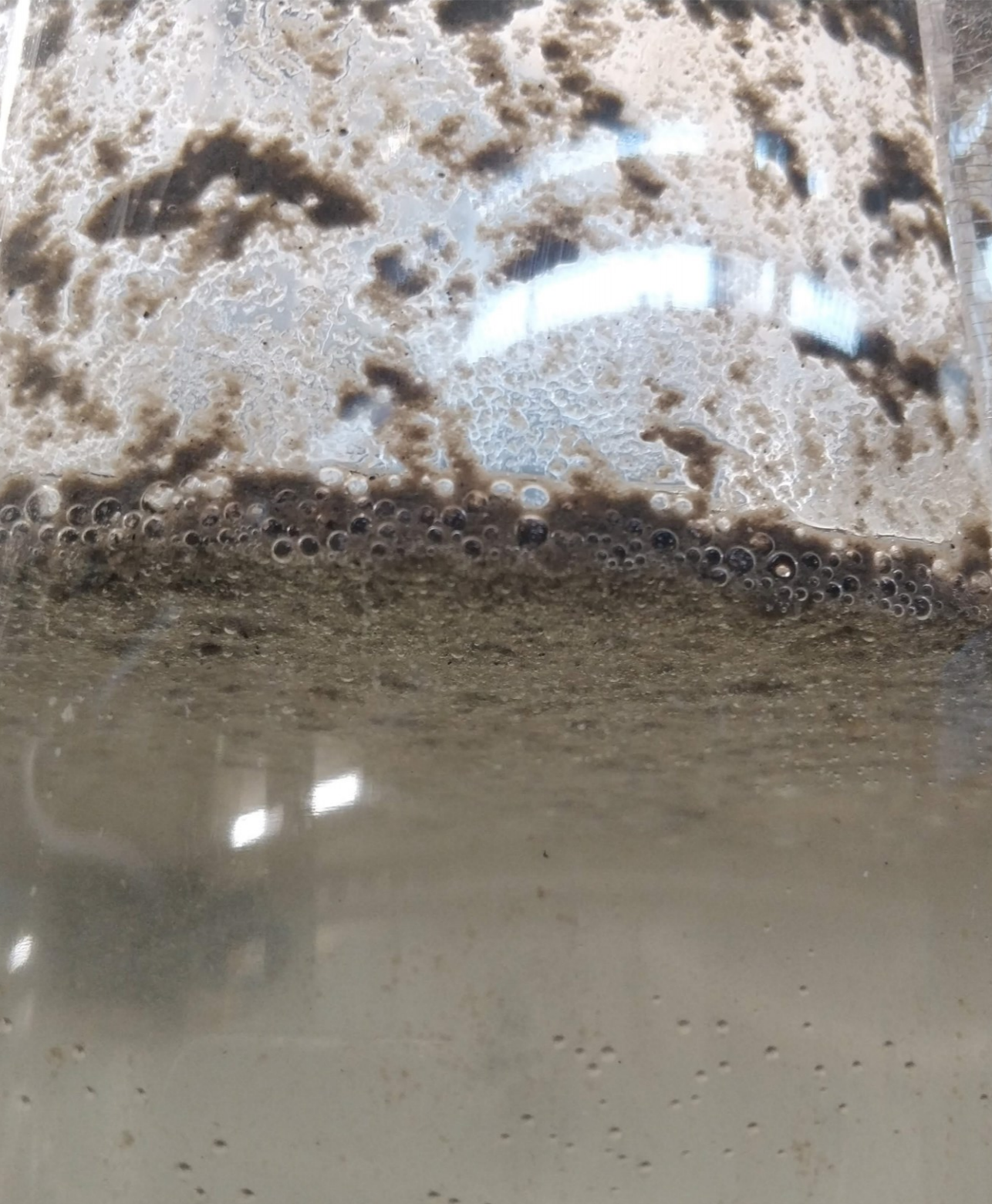
Concentrated suspended solids layer on the lab-scale DAF.
