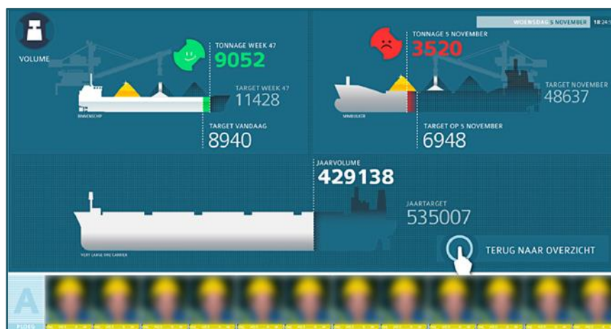
Figure 6. Detailed information about production targets on the screen of the galvanizing department. A full ship indicates that the target is met. In the top-left, tonnage of steel produced in a particular week, the ship on the top-right depicts the monthly production, and the bottom ship shows the yearly production.
