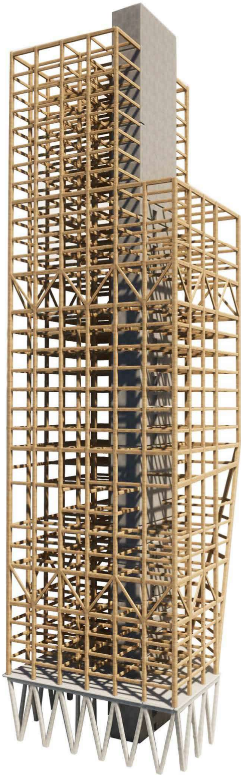
————— Glulam post and beam structure
