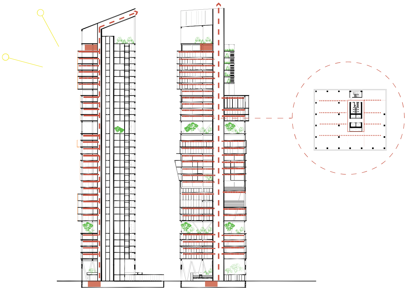
Mechanical ventilation with heat recovery
