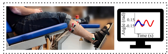
Fig. 1. Experimental setup. The subject was seated on an adjustable chair with their right foot attached to the dynamometer. The dynamometer perturbed and measured subject's right ankle joint angle and torque during a joint angle tracking task. A monitor provided real-time visual feedback on the angle target (in red) and the subject's ankle angle (in blue). EMGs of five leg muscles were recorded using disc-shaped Ag/AgCl electrodes in a bipolar configuration. (For interpretation of the references to color in this figure legend, the reader is referred to the web version of this article.)
