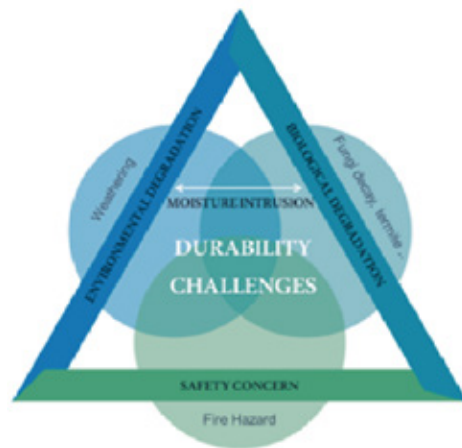
Fig 7: Durability challenges of mass timber in buildings and constructions (Ayanleye, S., Udele, K., Nasir, V., Zhang, X., & Miltz, H. 2022)
