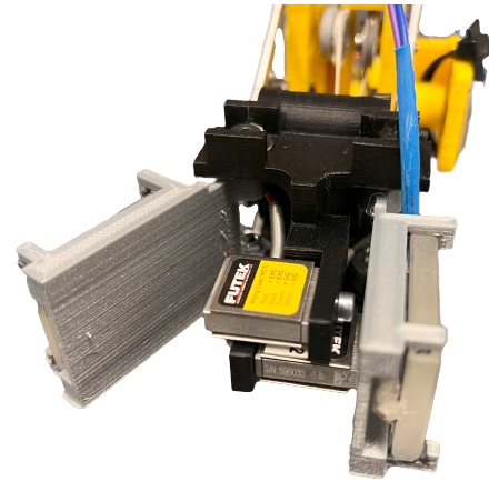
Fig. 2. Full assembly of the experimental setup. a) The grasping object. b) The friction modulation plates. c) The constant force system. d) The elbow support.
