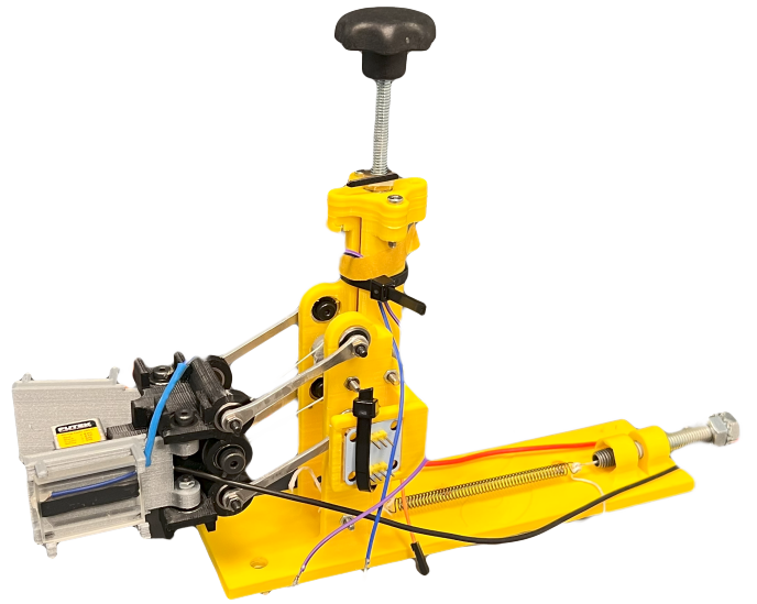
Fig. 5. Constant force system. The cylindrical structure houses a lead screw system, which adjusts the vertical force it provides. The screw at the lower-left corner connects to the pulley system and is used to adjust the pre-tension of the spring.
