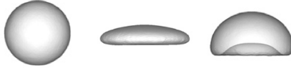
Figure 3: Bubble shapes from left to right spheres, ellipse and spherical cap. [32]
