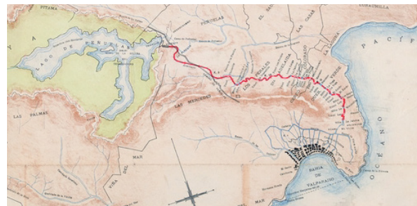
1901 drinking water project for Valparaíso showing the location of the reservoir and vicinity to Valparaíso
