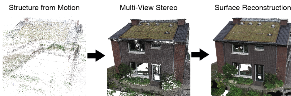
Figure 2: Sparse pointcloud, dense pointcloud and mesh (poisson)
