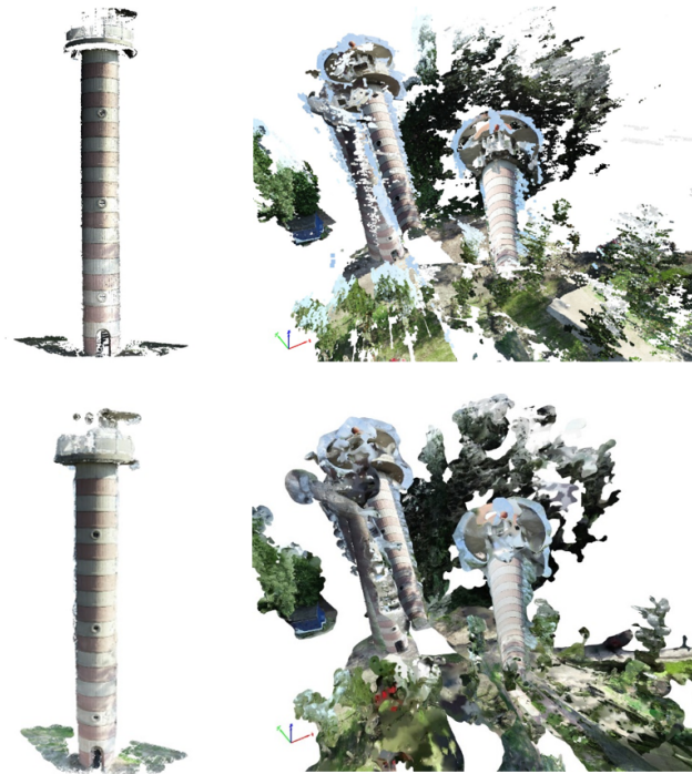
Figure 5.7: Comparison results with Pix4Dmapper. (Upper left: Point cloud generated by our software; Upper right: Point cloud generated by Pix4Dmapper; Lower left: Mesh generated by our software; Lower right: Mesh generated by Pix4Dmapper).
