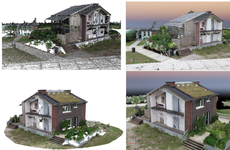
Figure 5.10: Comparison results with Pix4Dmapper. (Upper left: Point cloud generated by our software; Upper right: Point cloud generated by Pix4Dmapper; Lower left: Mesh generated by our software; Lower right: Mesh generated by Pix4Dmapper).
