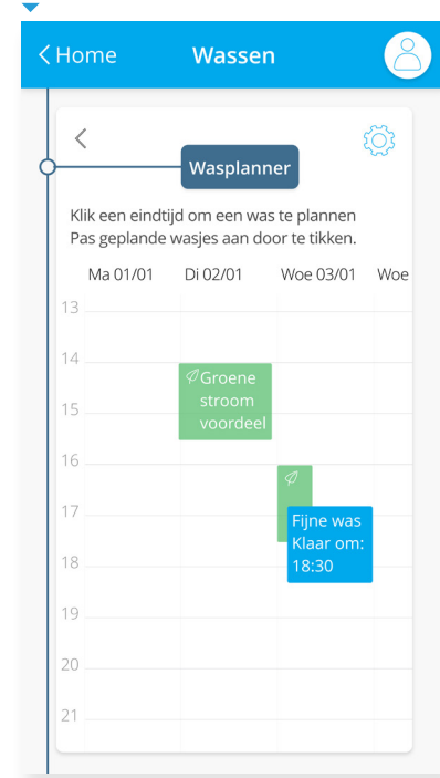
Figure 8.2-20: Green forecast of abundant renewable energy. Blue blocks are planned laundry tasks.
