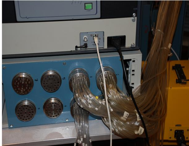
Figure A.4: Pressure scanner connected with tubes from surface pressure taps on the X-400 wing-flap configuration model
