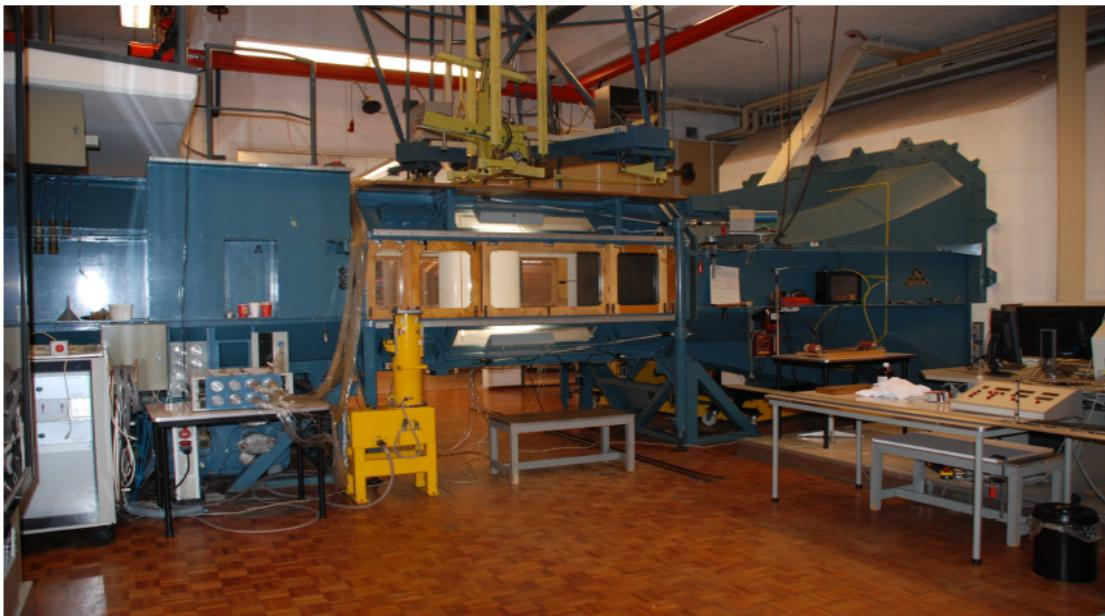
Figure 3.2: Low-Speed Low-Turbulence Wind-tunnel test section area overview [9]
