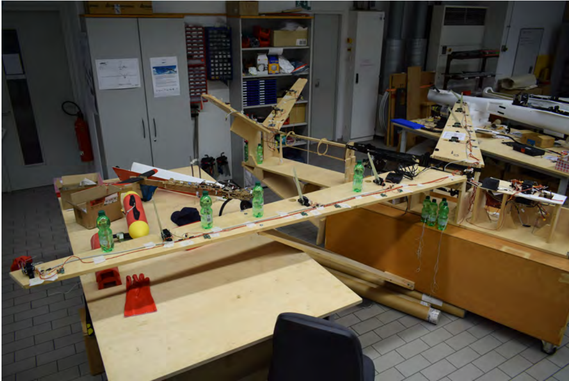
Figure 41. Wooden mock-up bench used for electrical system compatibility testing
