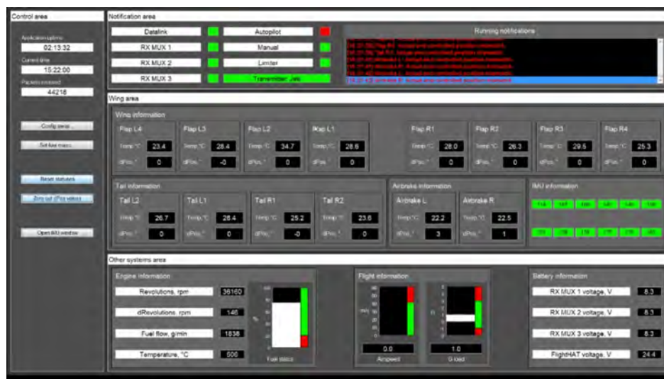
Figure 21. EDL main window during a taxi test
