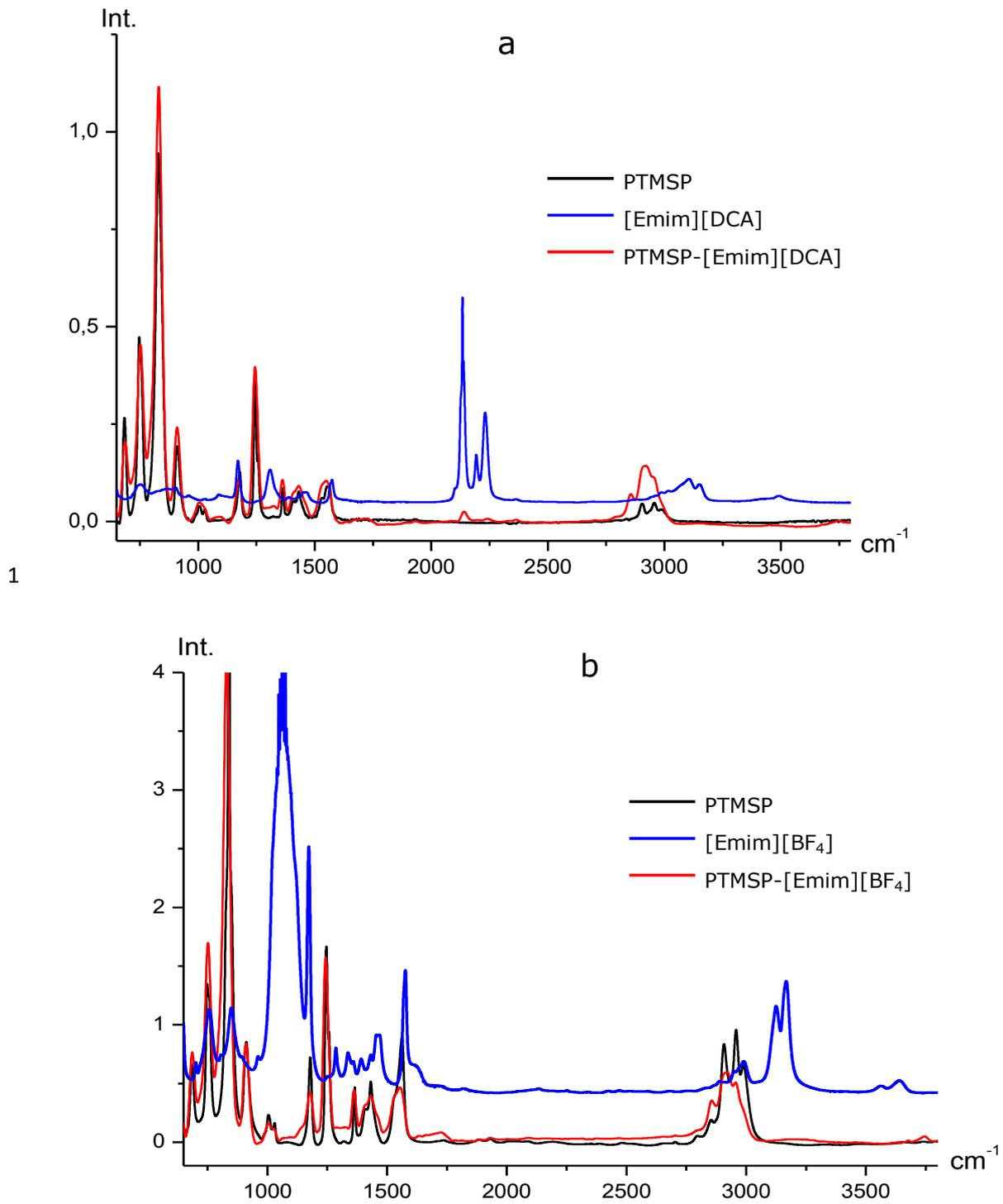
**Fig. 3.** FTIR spectra of swollen film of PTMSP in ionic liquids: [Emim][DCA] (a) and [Emim][BF<sub>4</sub>] (b). Spectra of pure PTMSP and individual liquids are also shown.
