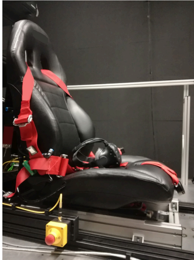
Fig 1. Active seat. The AS mounted on the motion platform with 6-point AB and Head-Mounted Display (HMD).
