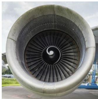
Figure 1.1: Aircraft engine nacelle installed with acoustic liners (in black) [2]
