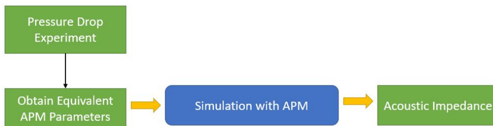
Figure 9.1: Methodology of APM simulations using the pressure drop experiments
