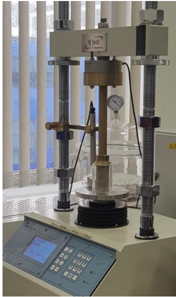
Figure 4: left: Brazilian Testing device. middle: white chalk sample after failure. right: grey chalk sample before failure
