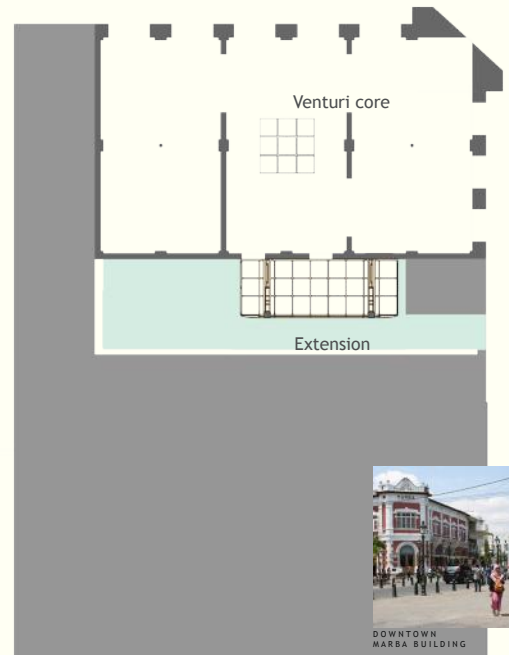
In the downtown version, a vertical flow pattern is made possible by the Venturi system. The small courtyard can cool down and freshen the incoming air.
