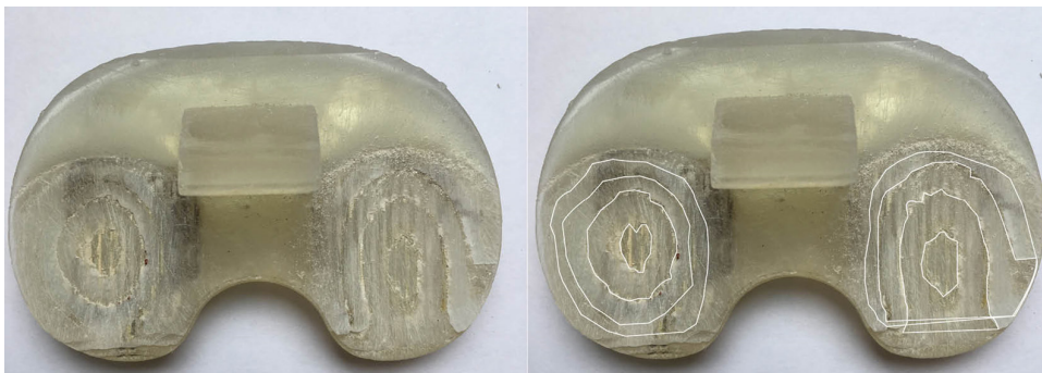
Figure 26 - Photo of insert when the third track on the left (lateral side) wore through. The white lines on the right contour the wear of the different layers.
