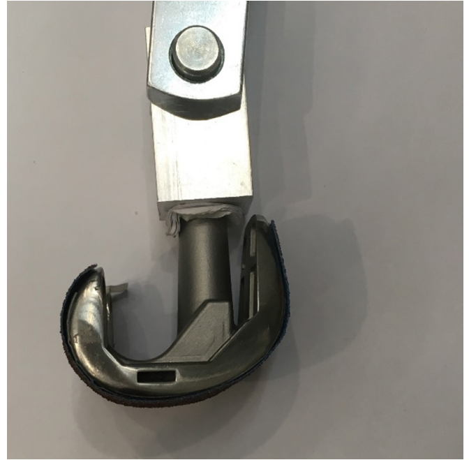
Figure 13 – Photo of the femoral head covered with sand paper. Left photo is the view from the front, and the right photo is the view from the side.
