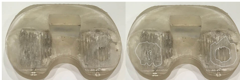
Figure 22 - Photo of insert when the second track on the right (medial side) wore through. The white lines on the right contour the wear of the different layers.
