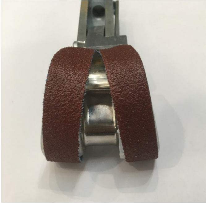
Figure 13 – Photo of the femoral head covered with sand paper. Left photo is the view from the front, and the right photo is the view from the side.
