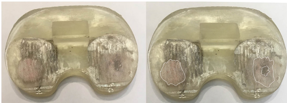
Figure 21 – Photo of insert when the first track on the right (medial side) wore through. The white lines on the right contour the wear of the different layers.
