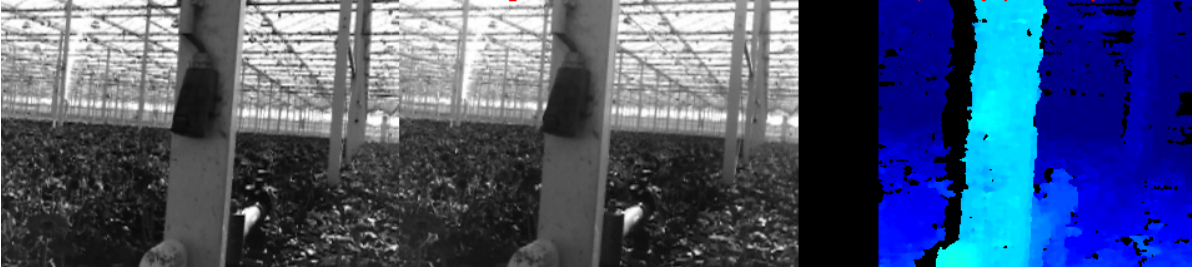
Figure 5.2: An example of occlusion. The image shows the left image, the right image, and the left disparity map, respectively
