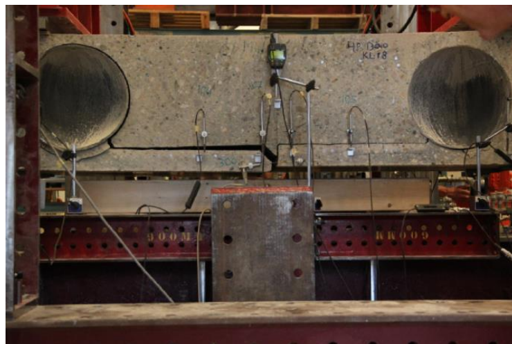
Figure 5.18: Brittle failure mechanism of bubble deck slab joint (Rijksoverheid, 2022)
