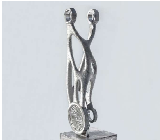
Figure 3: Example of generative design, an optimized robotic arm 3D printed using DED (WAAM) [5]
