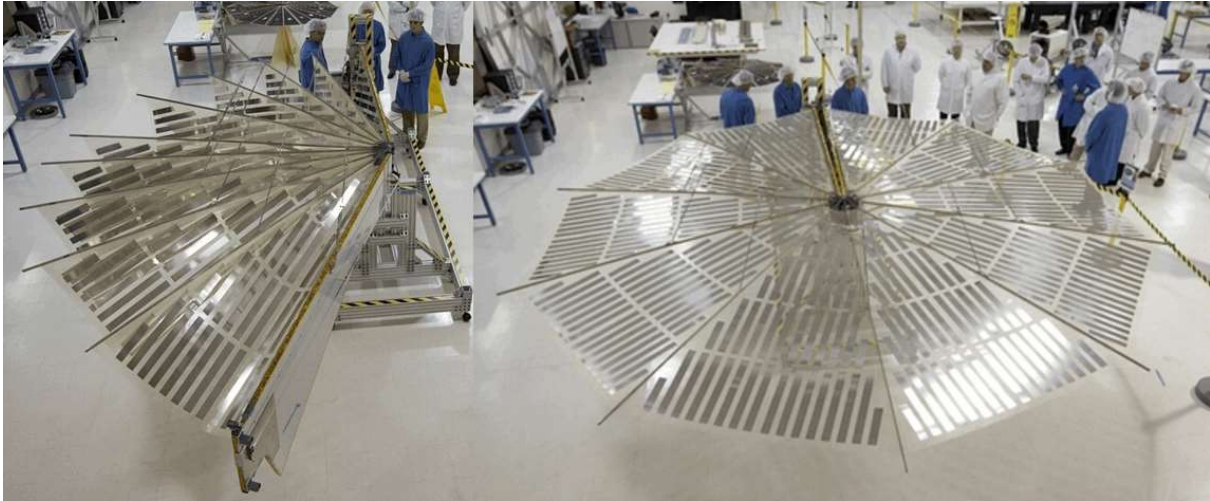
Figure 10: UltraFlex solar array by NASA and ATK during deployment (left) and fully deployed (right) [31]
