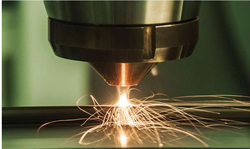
Figure 4: Powder-based DED scattering of particles [10]
