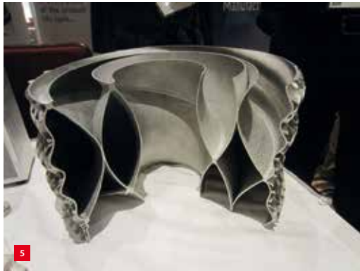
5 Optimised heat exchanger manufactured with additive help.
