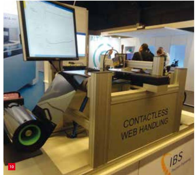
9 A stainless steel bellow with individually-welded rings, produced by BOA Nederland. 10 A web transport mechanism with porous air bearings, designed and manufactured by IBS.
