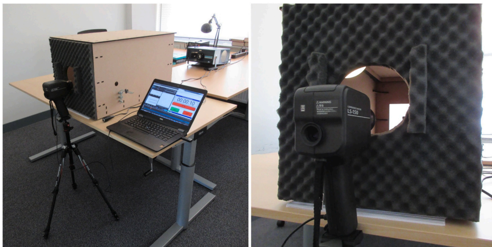
Fig. D6. Measurement configuration for recording luminance of the rear projection screen (Measurement series 3).
