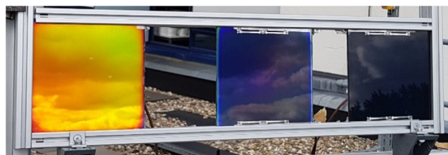
Figure 18. Temperature measurements of a colored mini module (orange, left), a mini module with an experimental filter (middle, outside of the scope of this work) and a standard mini module (right).
