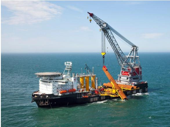
(c) Heavy Lifting Vessel Oleg Strashnov, Seaway 7, upending a Monopile[46]
