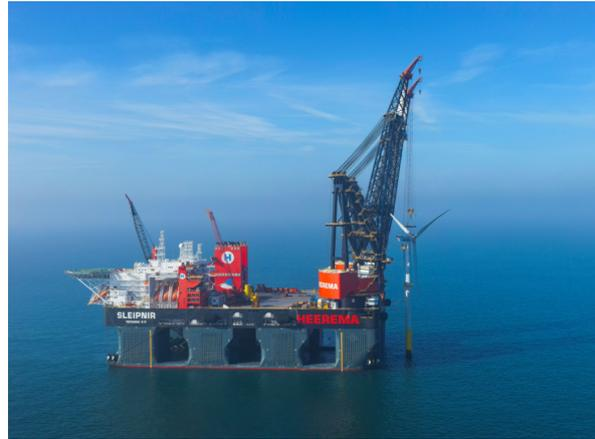
(d) Semi-Submersible Crane Vessel Sleipnir, Heerema, installing XXL turbine of DOT and TU Delft [11]
