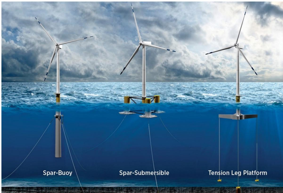
Figure 1.5: Graphical overview of floating foundations for offshore wind turbines [19]
