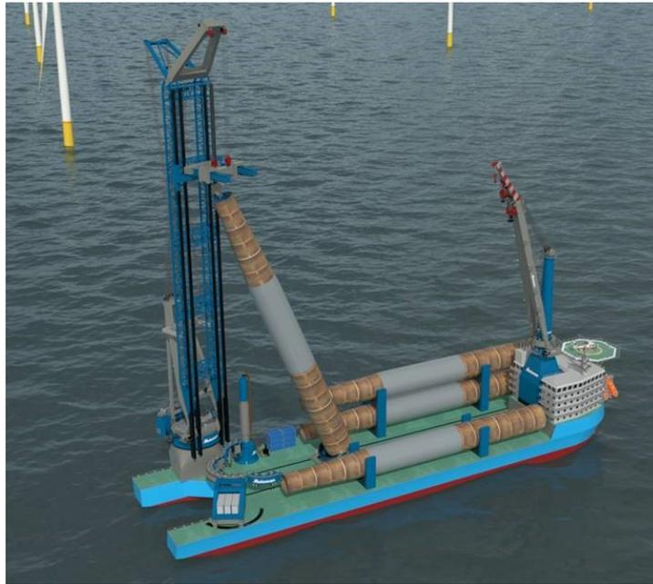
Figure B.4: A double trolley system for a fully constrained upending of the MP presented on the concept vessel Zephyr from Huisman
