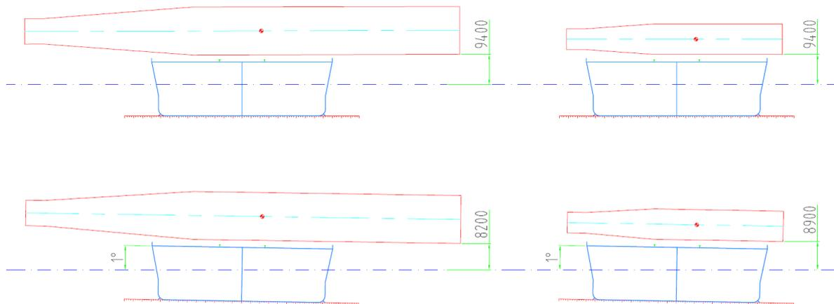
Figure C.1: Indication of reduction of air gap for a Roll angle of  $1^\circ$  for both MP XXL and MP Small
