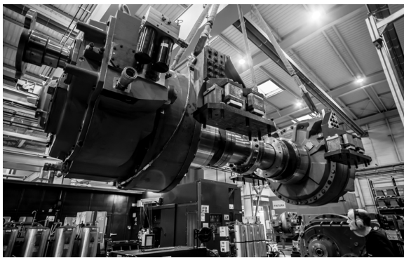
Figure 2. Lift operation of two gearboxes.
