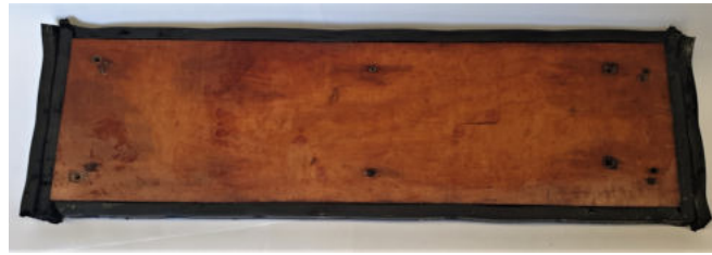
Figure 4.15: Plywood that was used as a vertical divider during perpendicular flow and a closing lid during parallel flow
