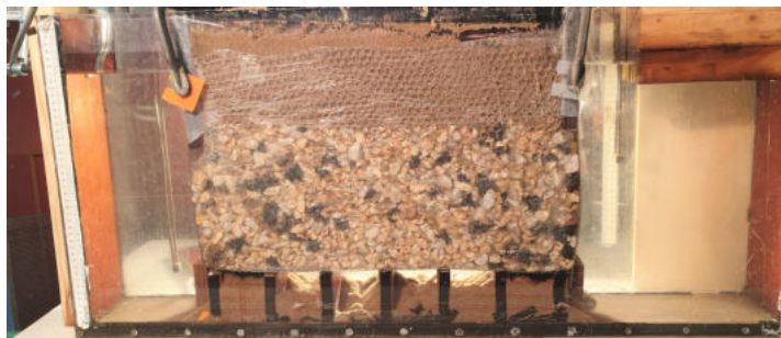
Figure C.10: A photo of the final model setup. The photo is taken after a long test which is why the boxed are filled with sediment
