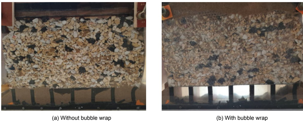
Figure 4.12: Initial infill of two similar tests with and without bubble wrap between the granular filter layer and the walls.
