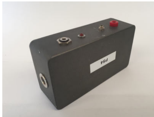
(b) Signal amplifier as used with the pressure sensors
