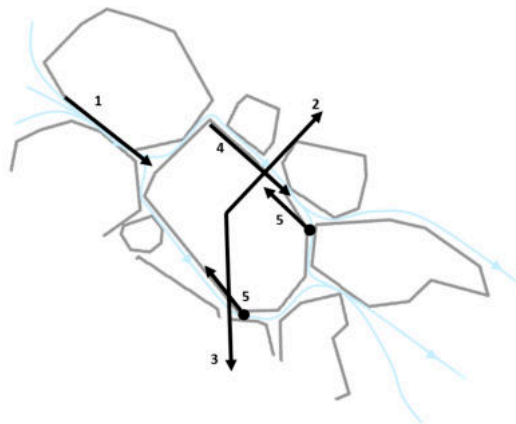
Figure 2.7: Forces on a grain, with: 1. Drag force, 2. Lift force, 3. Gravitational force, 4. Shear force, 5. Normal force.
