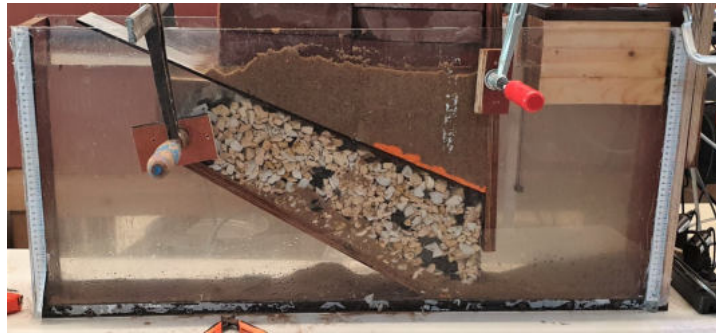
Figure C.6: A photo of the third model setup. What can be seen that the interface between the sand and the filter layer has been closed prior to the placement of the sand.
