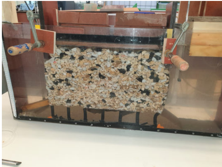
Figure C.8: A photo of the fourth model setup. In this setup there was no bubble wrap in place, which cause the large erosion
