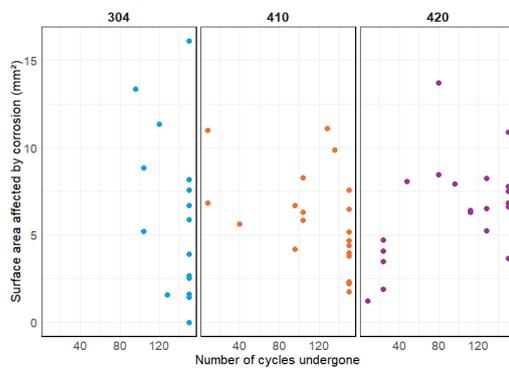
Figure 23: Scatter plot of surface area affected by corrosion against cycles completed under Continuous Sanizyme Reprocessing, with type 420 consistently exhibiting larger affected areas, particularly in earlier cycles, reinforcing its increased susceptibility.
