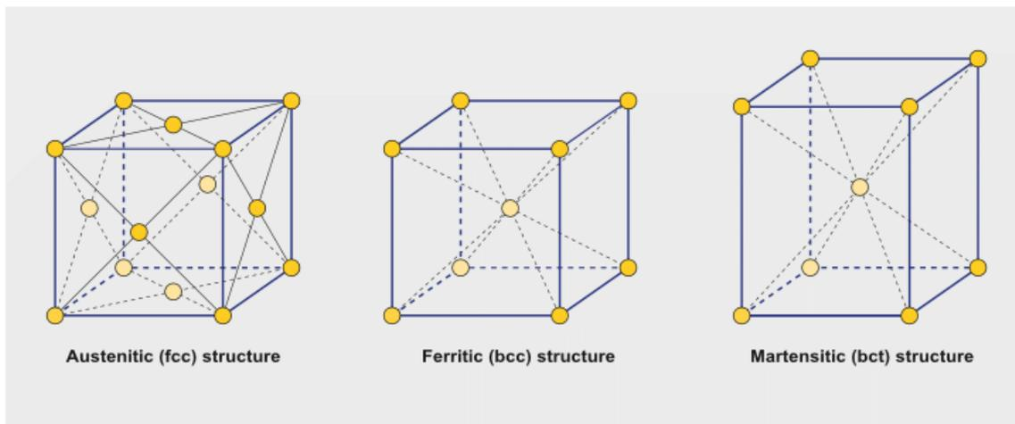
Figure 4: Crystal structures of Austenitic, Ferritic, and Martensitic stainless steels [29]
