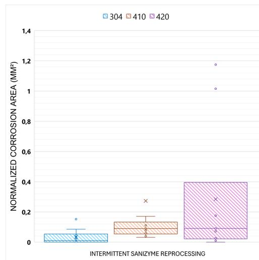
Figure 30: Box plot of normalised surface area affected per cycle under Intermittent Sanizyme Reprocessing, with type 420 exhibiting a larger median affected area per cycle, highlighting its heightened susceptibility.
