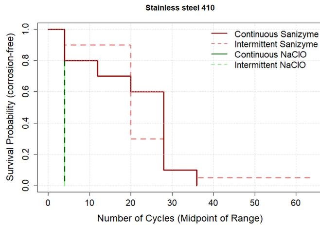
Figure 33: Kaplan-Meier survival curves for stainless steel type 410 comparing Continuous and Intermittent NaClO and Sanizyme reprocessing.
