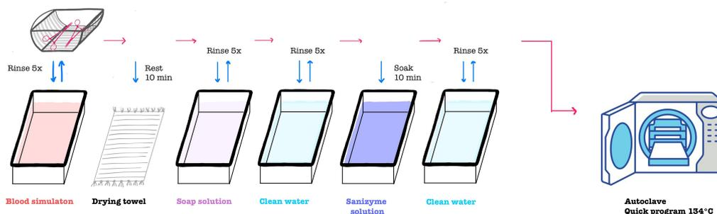
Figure 11: Setup of Continuous Sanizyme Reprocessing
