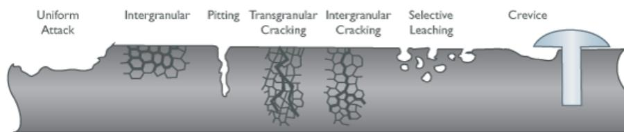
Figure 7: Forms of corrosion that affect stainless steels used in surgical instruments [9].
