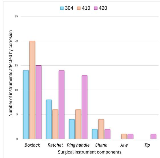
Figure 22: Component-specific corrosion distribution under Continuous Sanizyme Reprocessing, showing that the box lock remains the most corrosion-prone part, while type 420 demonstrates the highest incidence of affected areas.
