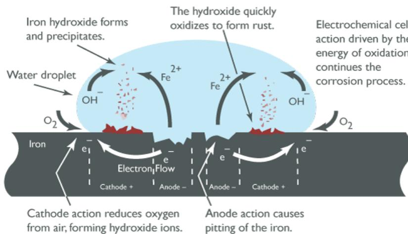
Figure 8: Oxygen concentration cell corrosion [46]
