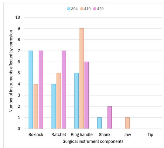
Figure 26: Corrosion distribution across instrument components under Intermittent NaClO Reprocessing, with the box lock and ratchet displaying the highest incidence of corrosion, particularly in type 420.
