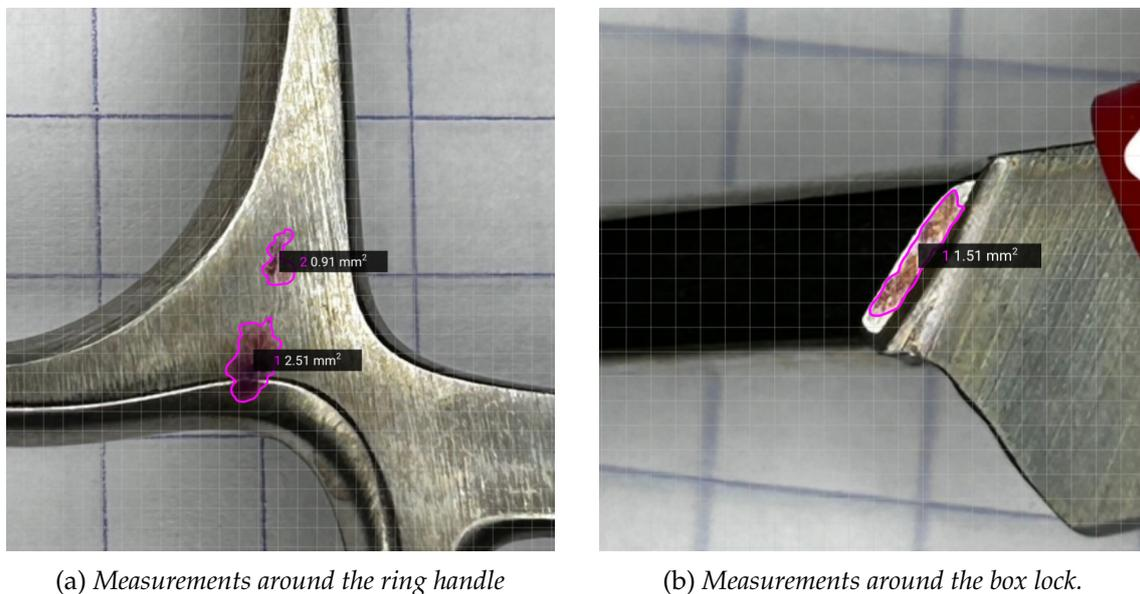
Figure 15: Measurements of surface area affected by corrosion using SketchAndCalc
