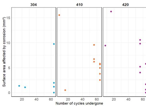
Figure 29: Scatter plot of surface area affected by corrosion against cycles completed under Intermittent Sanizyme Reprocessing, where type 420 demonstrates larger affected areas in earlier cycle stages, underscoring its increased susceptibility.
