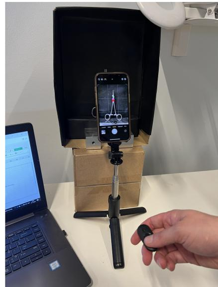
Figure 41: Photo booth setup used for documenting corrosion spots.
