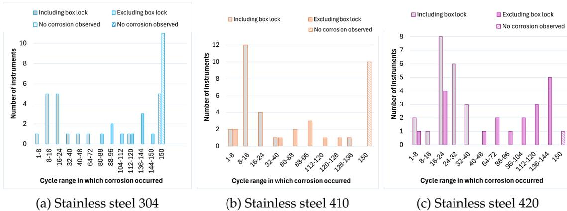
Figure 21: Corrosion onset in cycles during Continuous Sanizyme Reprocessing, comparing instruments with and without the box lock. Including the box lock significantly lowers the corrosion onset threshold across all materials, with type 410 exhibiting the most substantial effect.
