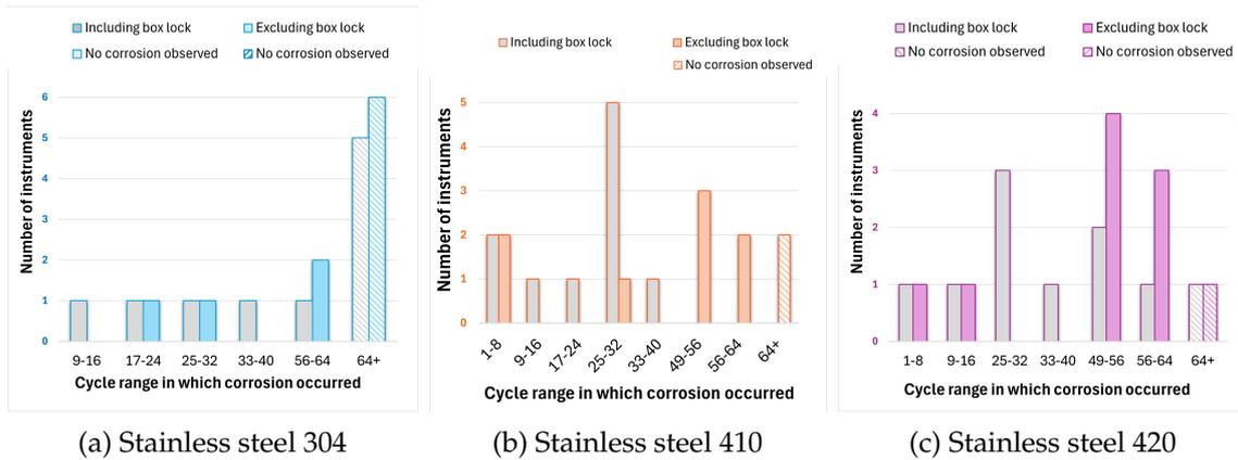
Figure 27: Number of cycles to corrosion onset across cycle intervals during Intermittent Sanizyme Reprocessing, comparing data with and without the box lock. Results indicate an earlier onset of corrosion in type 420, particularly when the box lock is included, highlighting increased susceptibility in this material.
