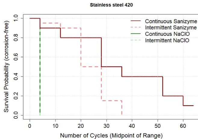
Figure 34: Kaplan-Meier survival curves for stainless steel type 420 comparing Continuous and Intermittent NaClO and Sanizyme reprocessing.
