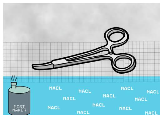
Figure 13: Schematic representation of the Salt Mist Test setup
