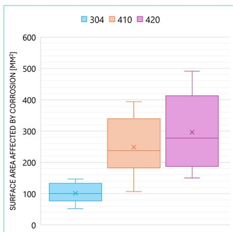
Figure 35: Box plot of surface area affected by corrosion following the Salt Mist Test, with type 420 showing the highest median affected area, underscoring its increased susceptibility relative to types 304 and 410.
