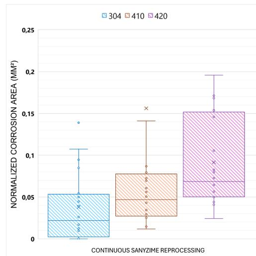
Figure 24: Box plot showing the normalised surface area affected per cycle under Continuous Sanizyme Reprocessing. Type 420 shows the highest median affected area, indicating a greater susceptibility than types 304 and 410.
