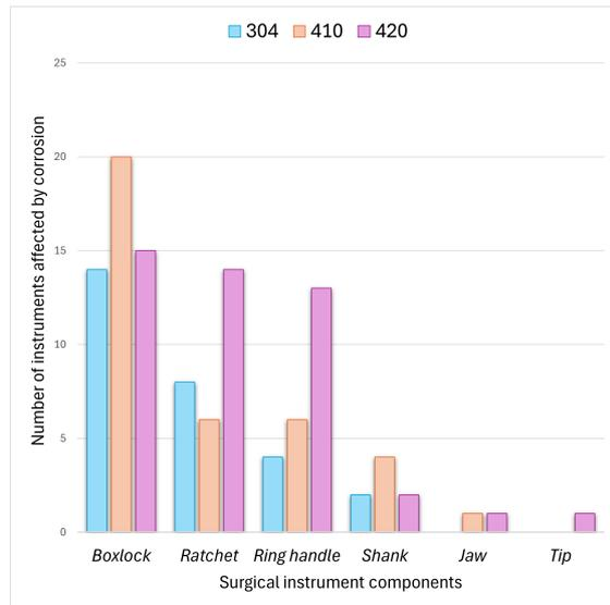
Figure 28: Distribution of corrosion across critical instrument components under Intermittent Sanizyme Reprocessing, with the box lock consistently showing the most vulnerability across materials. Type 420 exhibits the highest corrosion incidence across multiple components.
