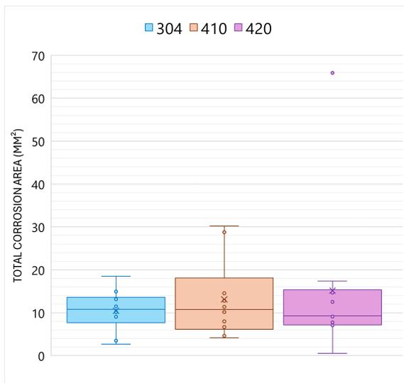
Figure 25: Surface area affected by corrosion following eight cycles of Intermittent NaClO Reprocessing, with type 420 demonstrating the greatest affected area, highlighting higher susceptibility to NaClO-induced corrosion.
