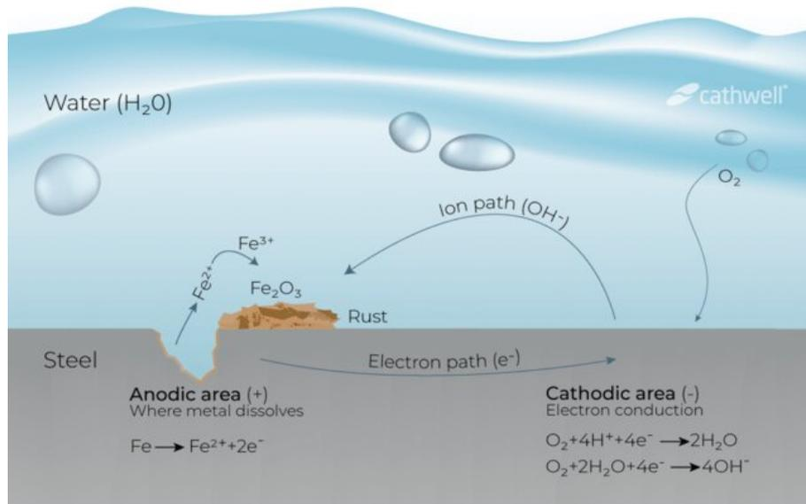
Figure 6: Electrochemical corrosion process in stainless steel, showing anodic and cathodic reactions that lead to rust formation [34].
