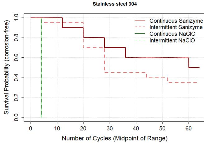
Figure 32: Kaplan-Meier survival curves for stainless steel type 304 comparing Continuous and Intermittent NaClO and Sanizyme reprocessing.
