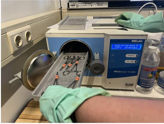
Figure 38: MELAtronic 15 EN+ autoclave used for sterilization.
