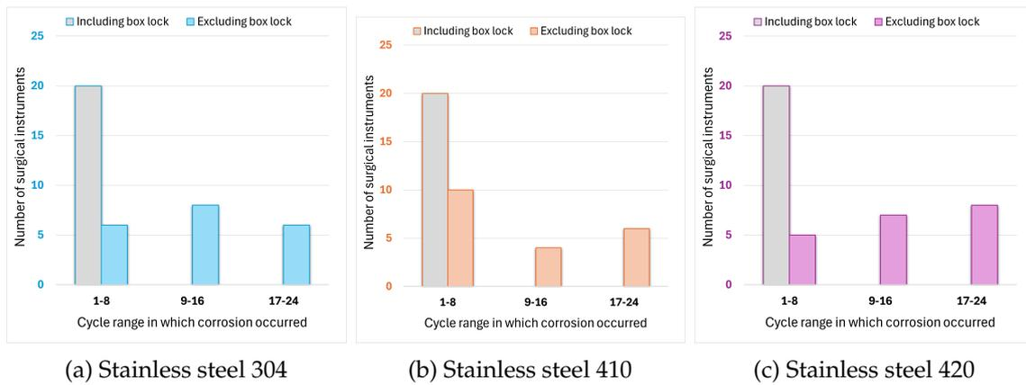
Figure 17: Number of surgical instruments exhibiting corrosion across cycle intervals (1-8, 9-16, 17-24), comparing results with and without the box lock. Results indicate an earlier onset of corrosion when the box lock is included for all stainless steel types, underscoring the susceptibility of the box lock region to early-stage corrosion.
