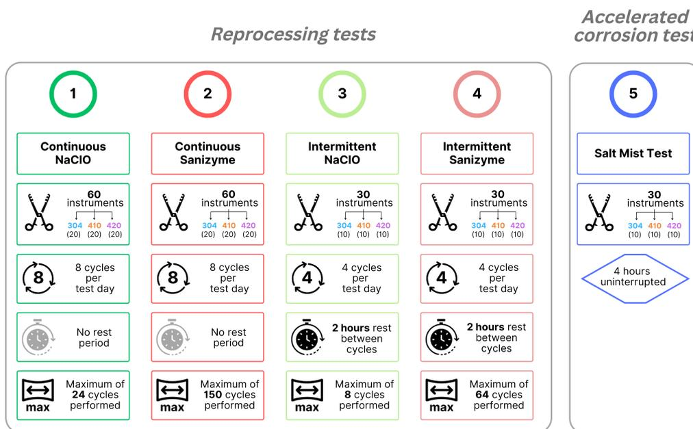
Figure 14: Overview of reprocessing and accelerated corrosion test protocols. The diagram summarises key parameters for each test.
