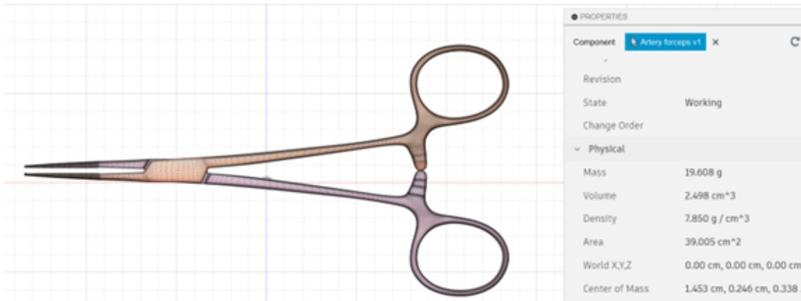
Figure 16: *Simplified CAD model of the forceps used to estimate total surface area (approx. 40 cm<sup>2</sup>) for comparative analysis of corrosion-affected regions.*
