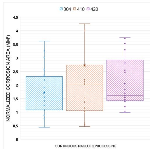
Figure 20: Box plot of normalised surface area affected per cycle, revealing that type 420 has the highest median affected area per cycle, indicative of heightened susceptibility under Continuous NaClO reprocessing.
