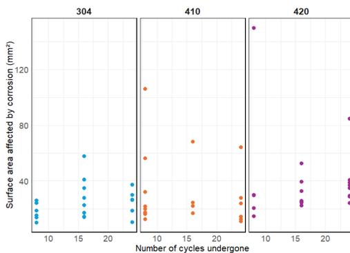
Figure 19: Scatter plot illustrating the relationship between total surface area affected by corrosion and cycles completed. Data points for type 420 show a general increase in affected areas with higher cycle counts, reflecting trends in corrosion progression over time.
