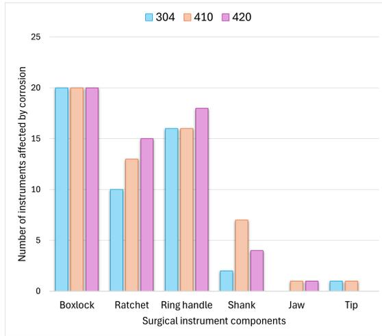
Figure 18: Distribution of corrosion across specific instrument components, with type 420 exhibiting the highest overall susceptibility. The box lock demonstrates the greatest vulnerability across all materials.
