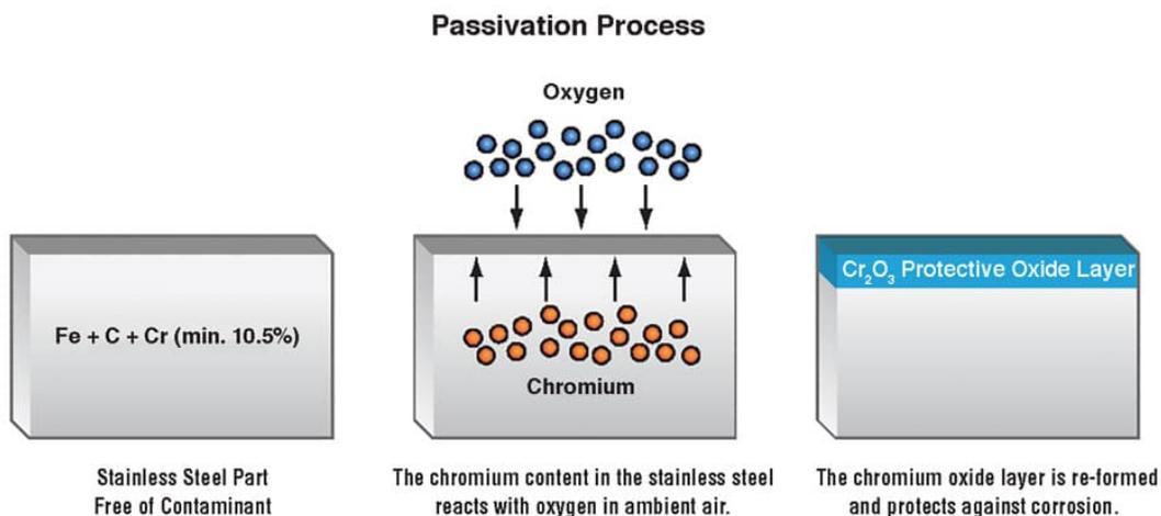
Figure 5: Illustration of the passivation process in stainless steel. Chromium in the stainless steel reacts with oxygen in ambient air to form a protective chromium oxide layer, which protects against corrosion [32].
