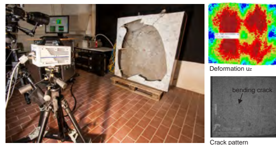
The façade after failure and results from optical measurement
