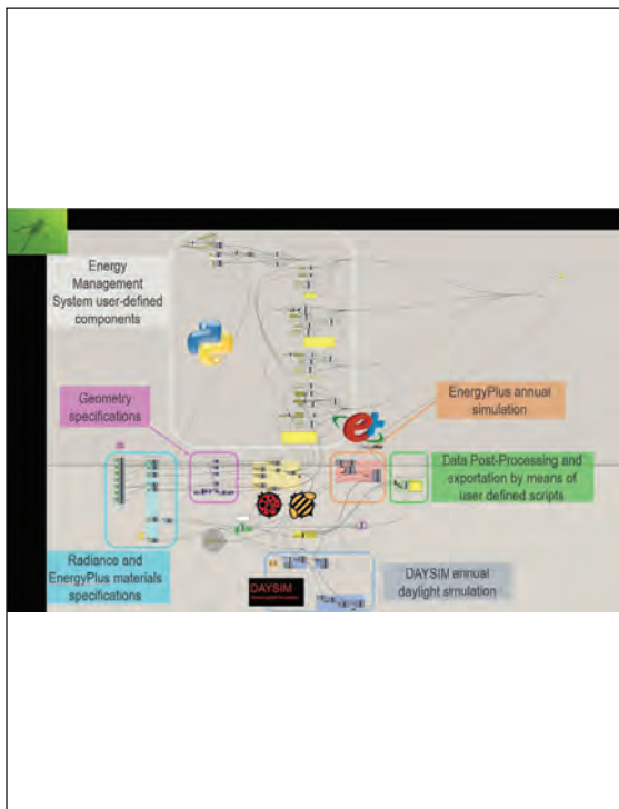
Fig. 1. The simulation tool created in Grasshopper with the indication of the different sections composing it and the software used in each of them
