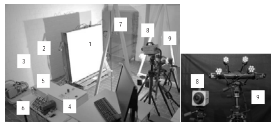
The developed test set-up: 1- specimen, 2- steel frame, 3- vacuum pump for wind load simulation, 4- controller, 5- measurement amp., 6- manometer, 7- safety glass, 8- high-speed camera, 9- 3D measurement system
