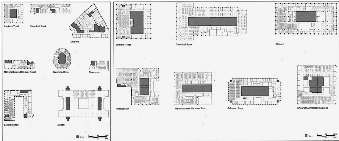
FIGURE 5.3. Comparative plans for trading floors in the United States and United Kingdom, designed by DEGW, 1986.
