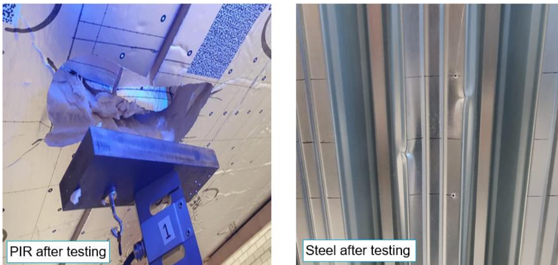
Figure 35 Failure of the PIR after testing (on the left) and the steel sheet after testing (on the right).
