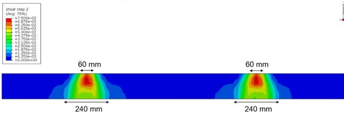
Figure 55 Shear stress at cross section cut under the load (LCA, step 2: load = 4000 N)
