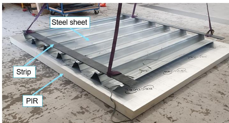
Figure 18 Lifting of the specimen (turned upside down).
