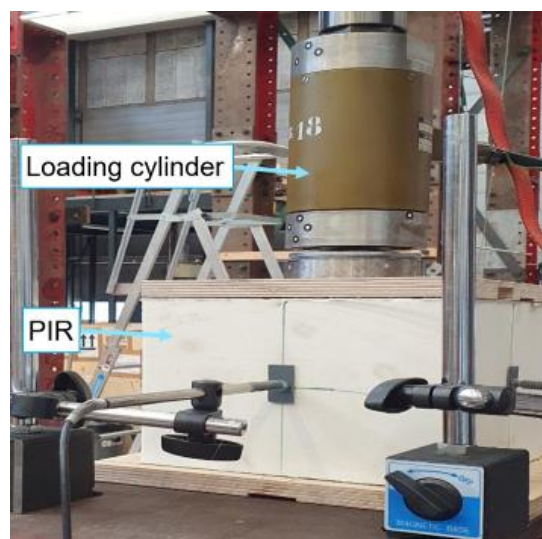
Figure 47 Compression test of PIR insulation.
