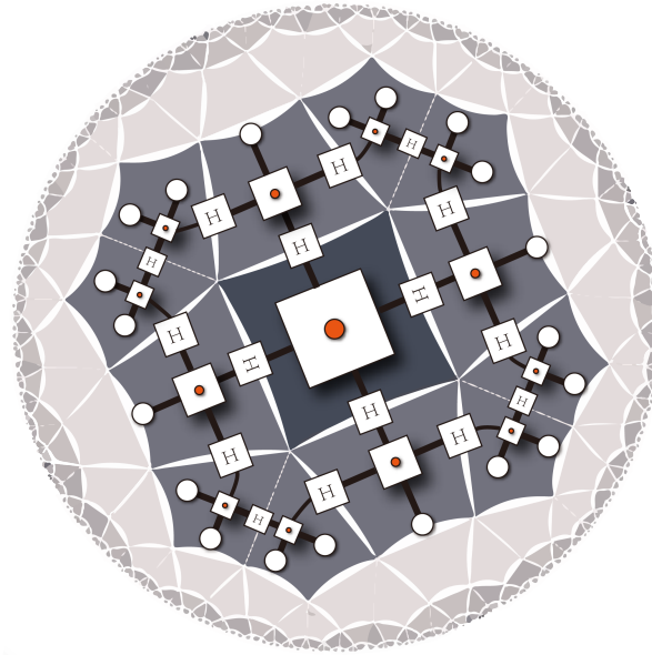
Figure 2.23: The [[4, 5]] HTN code at L = 1 [92], following the vertex inflation rule.
