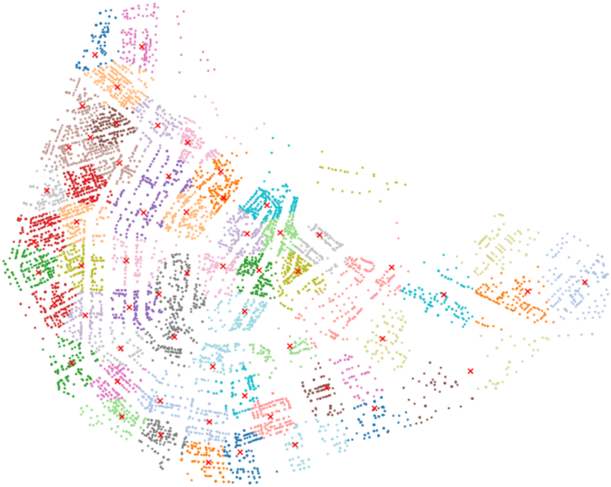
Figure 7.1: The buildings in the center of Amsterdam divided into 60 clusters by k-means
