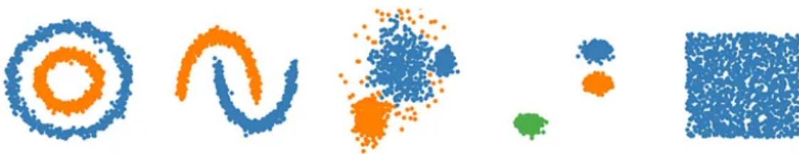
Figure 5.4: The performance of DBSCAN on various point sets (Andrewngai, 2020)
