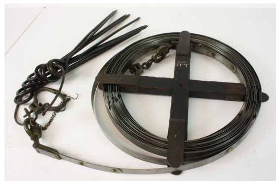
Measuring chain used for determining verponding (land tax) "made of sections of galvanized iron or steel wire, 3 to 4 millimeters thick. The ends of the sections (links) are fitted with eyes and linked together with rings." 1850-1900 (Rijksmuseum Boerhaave)
