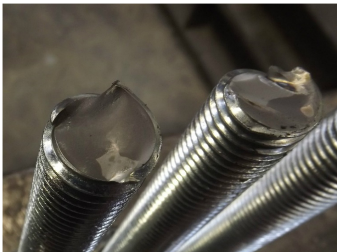
Fig. 15. Failure surface of bolts (P3.2-1).
