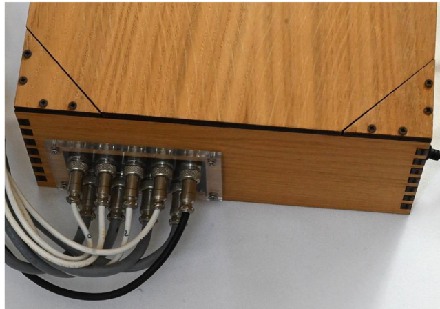
Fig. 12. The pin connectors on the box for the electronics. On the right the USB cable connection to the laptop.
