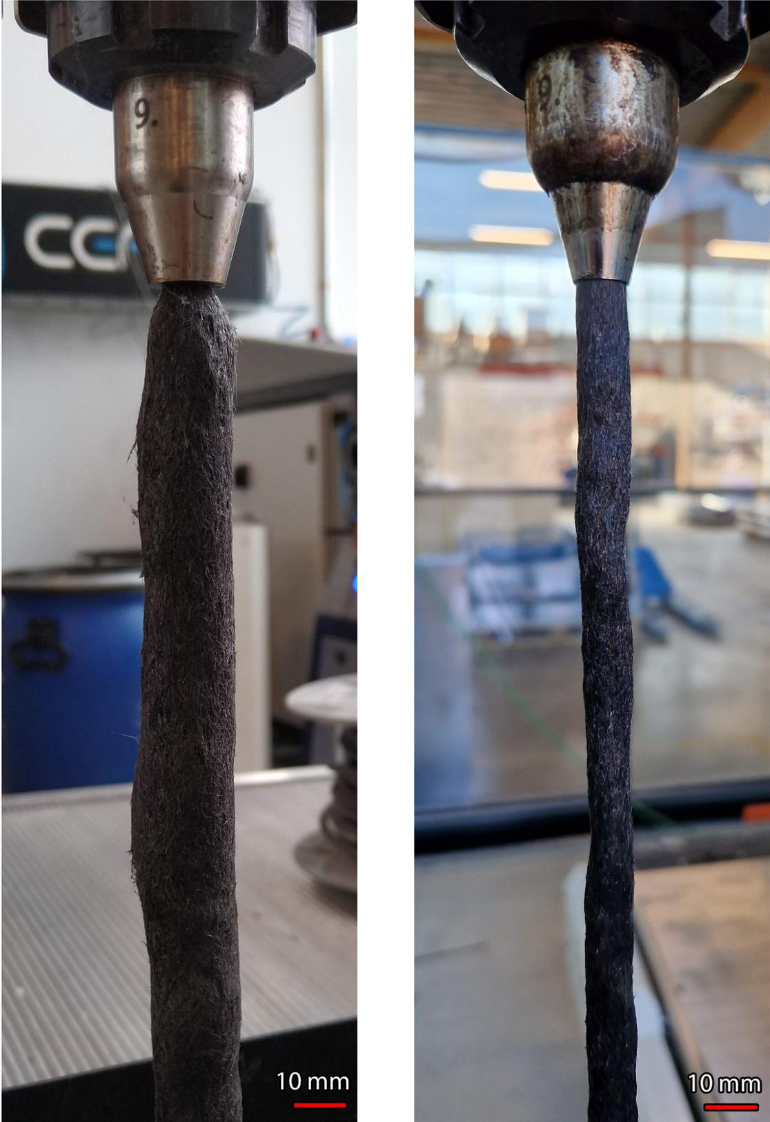
(a) Original 11 mm long fibre extrusion showing a high degree of swelling
