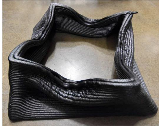
**Figure 2.4:** Large-scale AM box print that has collapsed due to overheating from printing too fast [17]
