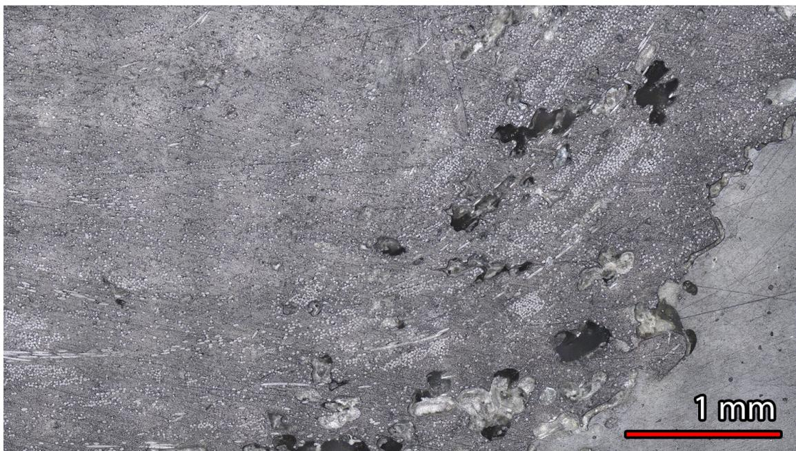
Figure 5.11: Sectioned microscopy of LGFPP/PE blend, showing un-dispersed fibre agglomerates
