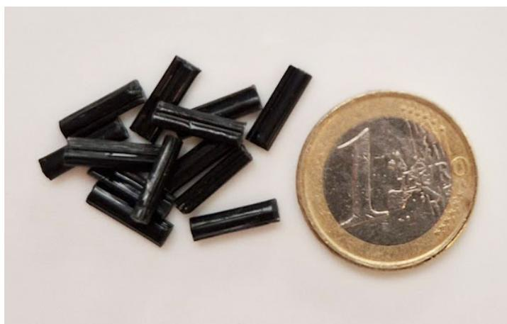
**Figure 3.3:** 11 mm LGFPP pellets, 1 euro coin for scale
