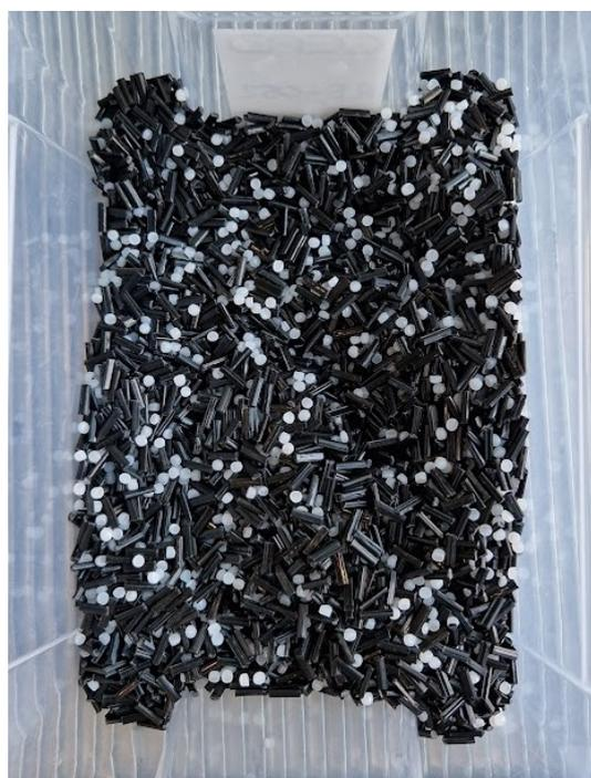
**Figure 5.1:** Mixed pellet input, black long glass fibre polypropylene pellets with lower temperature melting white HDPE for lubrication
