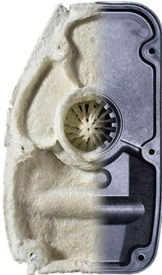
**Figure 4.7:** Injection moulded long fibre thermoplastic part, with fibre 'skeleton' visible on the left, exposed by pyrolysis <sup>1</sup>
