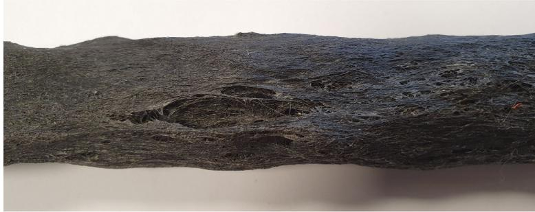
**Figure 2.12:** 12 mm fibre pellet extrusion test, showing fibrous exterior and large cavity caused by fibre/matrix separation from swelling
