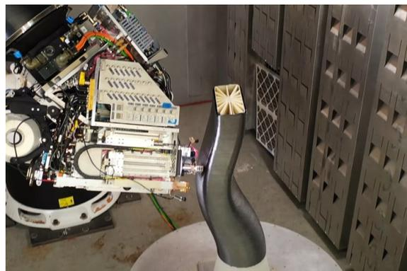
(b) SCRAM fibre over-wrapping on top of 3D printed scaffold
