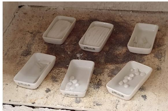
(b) Samples after calcination, the resin has been removed, revealing bare glass-fibres
