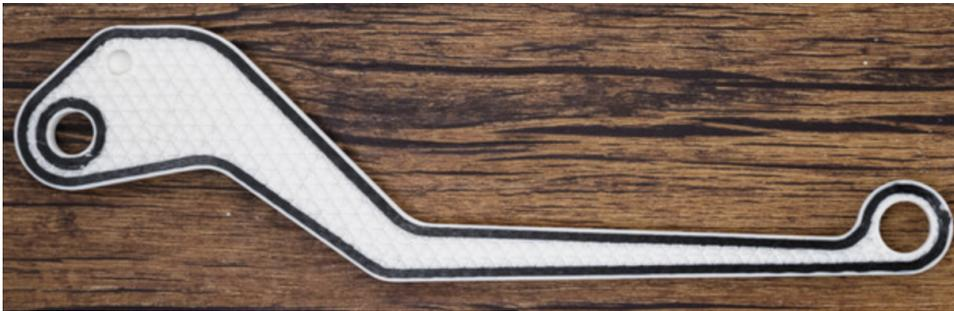
**Figure 2.5:** Markforged 3D printed part with white nylon, reinforced by continuous black carbon fibre reinforcement
