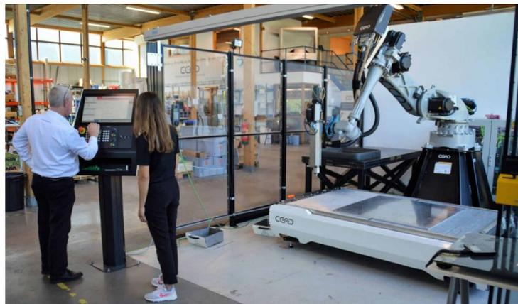
(b) CEAD Large-scale Additive Manufacturing printer<sup>1</sup>
