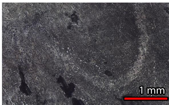
Figure 5.10: Sectioned microscopy of LGFPP/PE blend, showing a white region of discrete unmixed HDPE inside darker PP
