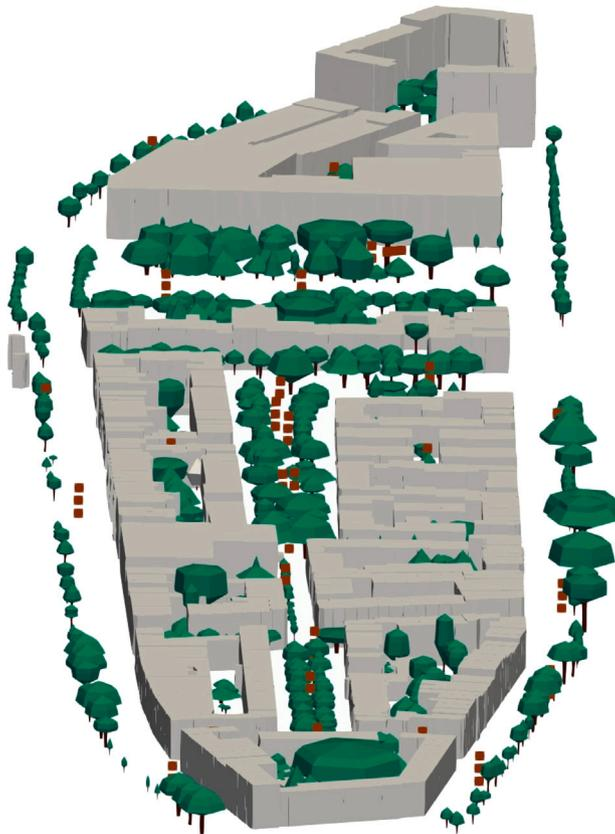
Fig. A.2. Probes used to compute grid convergence index. Grey: buildings, green: trees, red: probes. (For interpretation of the references to color in this figure legend, the reader is referred to the web version of this article.)
