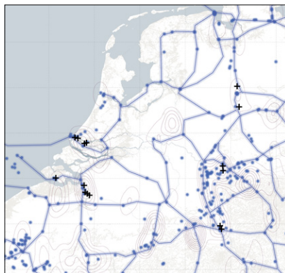
F. 30 Existing high tension cables
