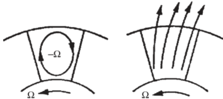
Figure 3.11: Relative eddy without through-flow (left), and relative flow at impeller exit (right)
