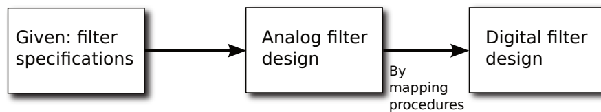
Figure 2.53: A two-step procedure for designing IIR digital filters.
