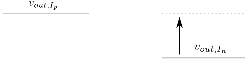
Figure 4.11: Positive I offset compensation. v_{out,I_n} is raised to the level of v_{out,I_p} .
